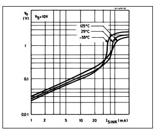
Figure 6 : Low Output Voltage versus Output Sink Current
