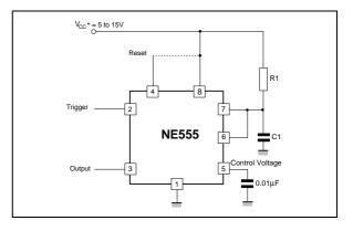
The circuit triggers on a negative-going input signal when the level reaches 1/3  $V_{CC}$ . Once triggered, the circuit remains in this state until the set time has elapsed, even if it is triggered again during this interval. The duration of the output HIGH state is given by  $t = 1.1 \ R_1 C_1$  and is easily determined by figure 12.
