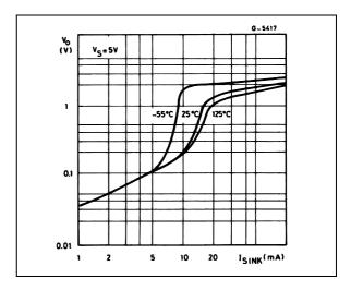
Figure 5 : Low Output Voltage versus Output Sink Current
