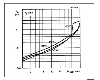
Figure 7 : High Output Voltage Drop versus Output
